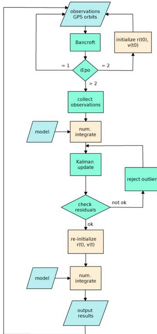
Initialization of the orbit, cycle slip fixing, ambiguity solution, and outlier rejection are all done in one processing step.
